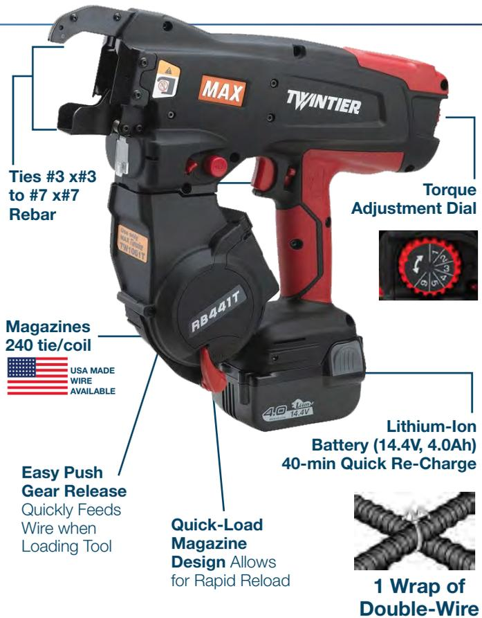
The TWINTIER is the newest edition to our Rebar Tier line. This model relocates the wire spool to below the jaws of the tool. **ADVANTAGE:** the wire is then fed through the tool and looped twice, to create a twin wire tie as opposed to the 3 wrapped single wire tie in previous models. In a single wrap the TWINTIER produces a stronger, **more secure rebar connection in 30% less time!**
